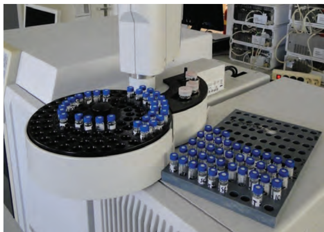
Fig. 1 Gas chromatograph mass spectrometer (GC-MS) in the Research Lab Molecular Epidemiology
