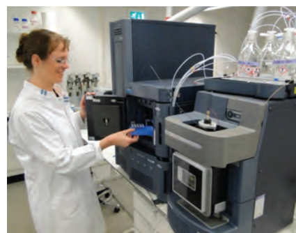
Fig. 5 UPLC system with tandem triple quadrupole mass spectrometer used for ultrasensitive detection of unique chemical signatures of xenobiotics in body fluids
