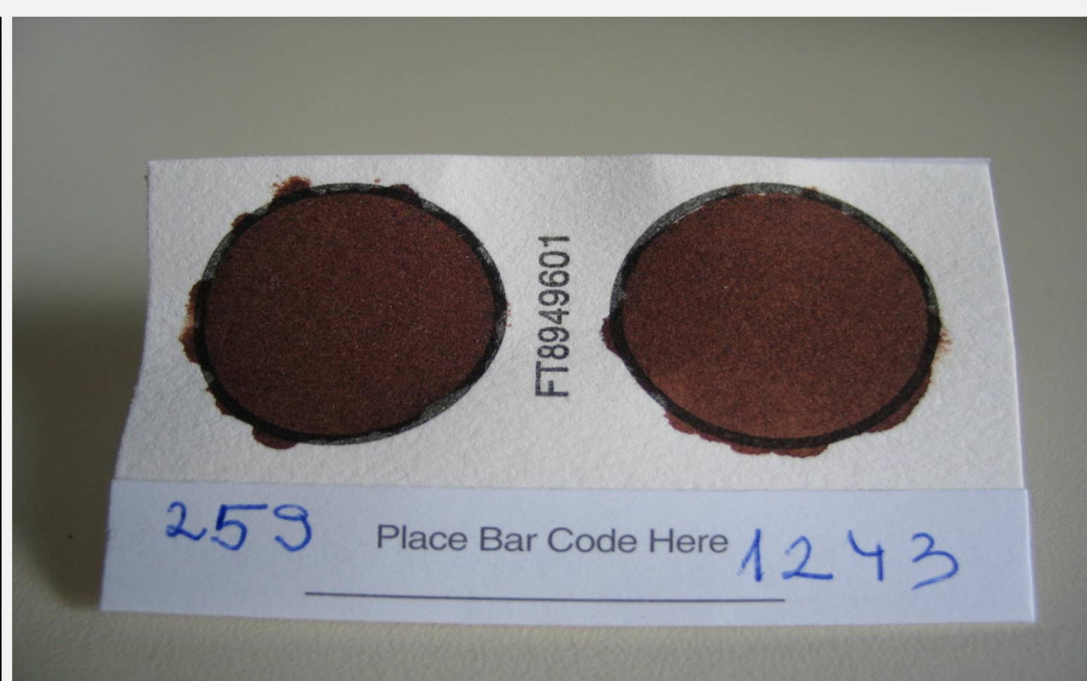
Figure 2. FTA Mini cards for collection, archiving and purification of nucleic acids from blood samples.
